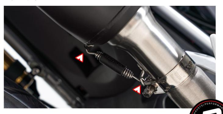
Install the supplied heat shield bracket onto the supplied heat shield clamp.
