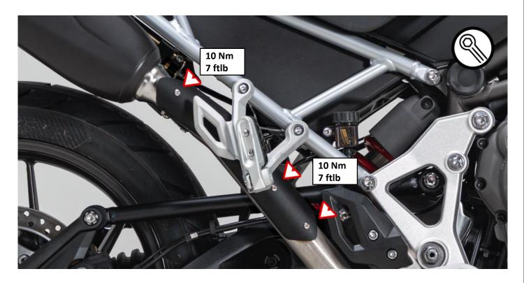
Align the REMUS sport exhaust and tighten the connections.
