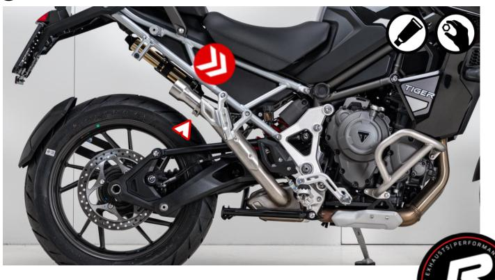
Slip on the REMUS sport exhaust onto the connection tube. Screw the bracket of the exhaust with the motorcycle.
