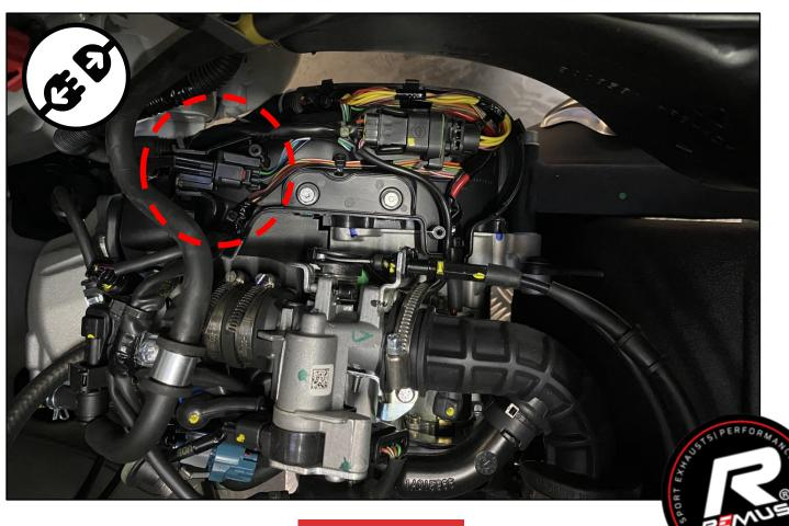
Carefully detach the O2 sensor cable from the plastic clips.
