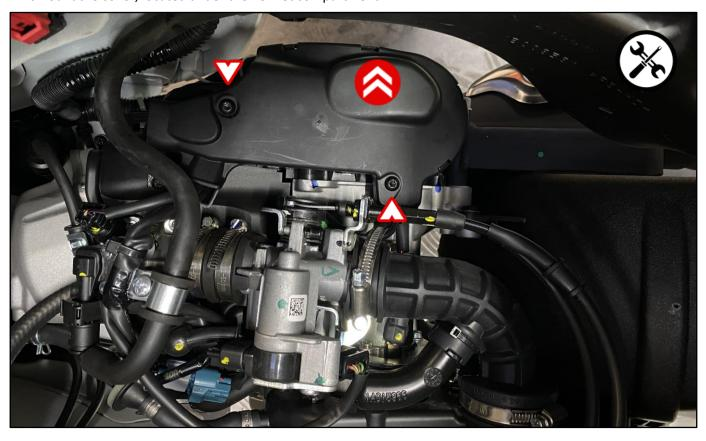
Disconnect the connector of the O2 sensor.
