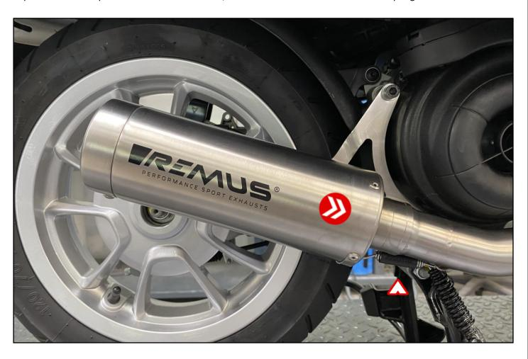
Align the REMUS sport exhaust and tighten the connections.
