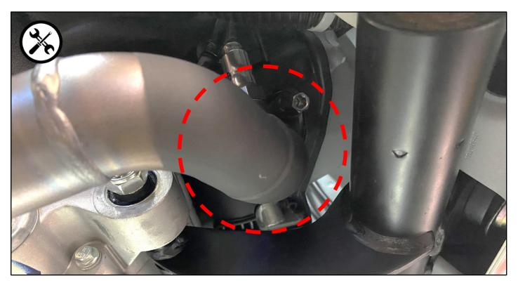
Loosen the bracket screws and remove the stock silencer.
