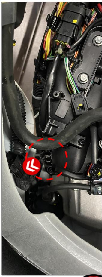
Loosen the flange connection of the header.
