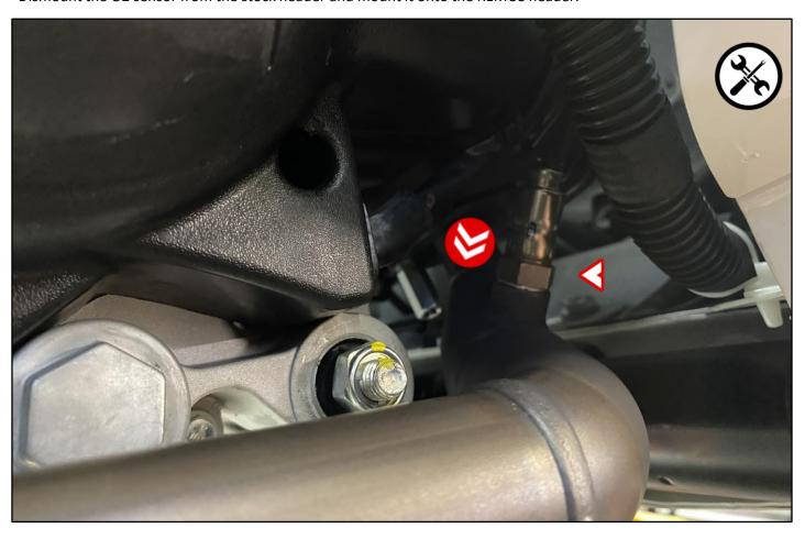
Reconnect the O2 sensor, fix the cable with the plastic clips and remount the plastic cover.
