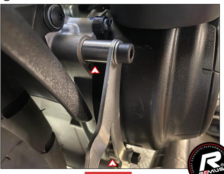
Slip on the REMUS sport exhaust onto the header, bold it with the bracket and hook the spring.
