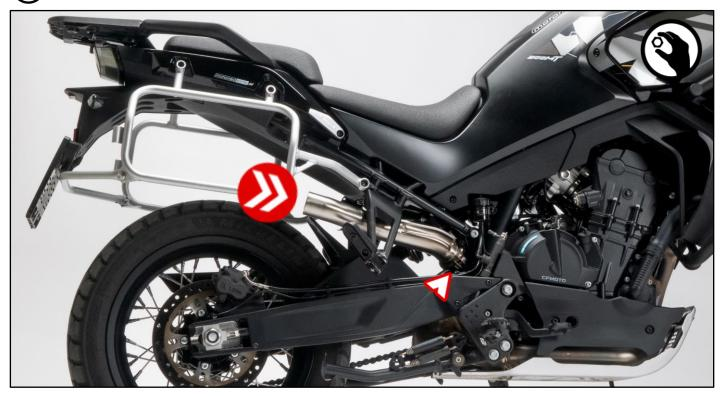
Slide the REMUS sport exhaust onto the connection tube and slightly tighten the bracket screw.
