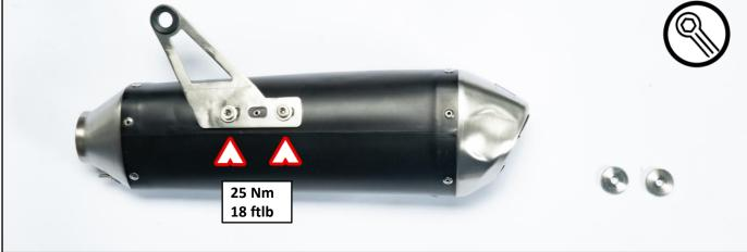
Mount the supplied spacers onto the bracket.
