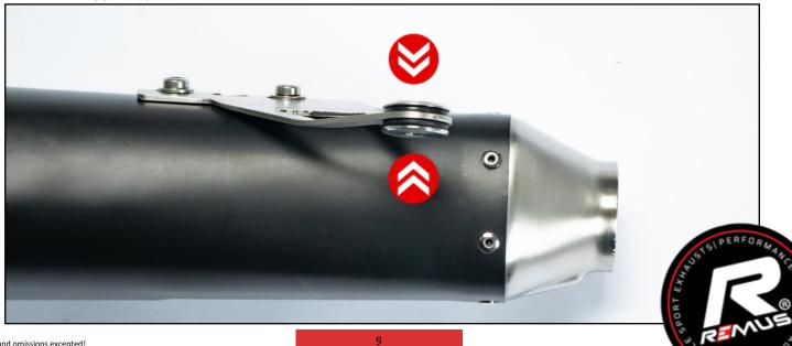
Install the REMUS connection tube, by using the serial clamp, onto the serial header.
