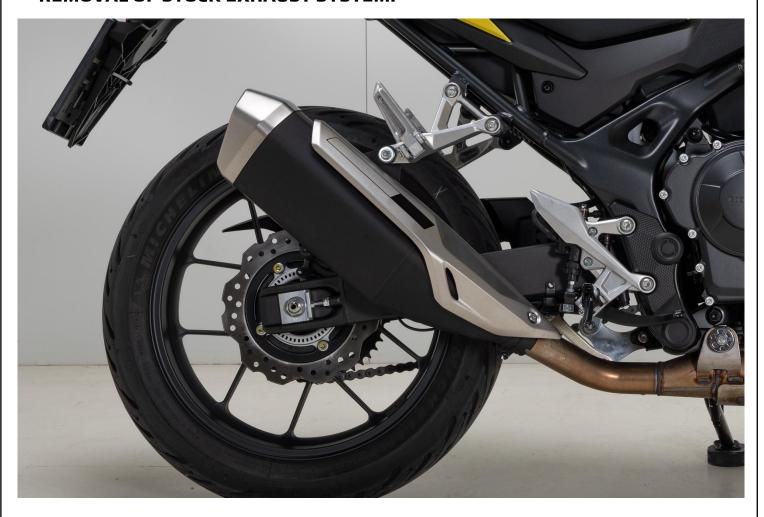
Dismount the heat shield. Loosen the screw of the bracket and the clamp and remove the serial mufflers.
