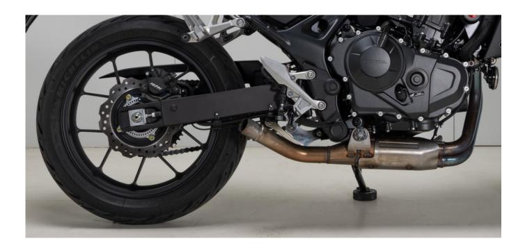
Mount the supplied clamp for the heatshield on the serial header Install the REMUS connection tube, by using the supplied clamp, onto the serial header.
