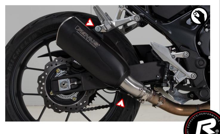
Align the REMUS sport exhaust and tighten the connections.
