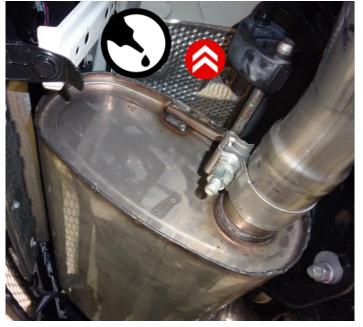
Install the two outlet tubes onto the REMUS sport exhaust. Slip On and mount the REMUS Tail pipes onto the outlet.
