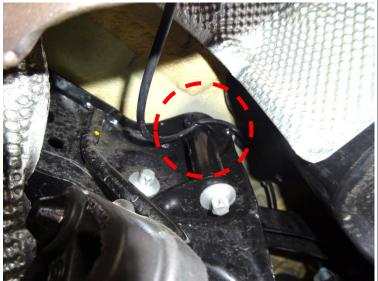
Connect the actuator cable with the REMUS actuator.
