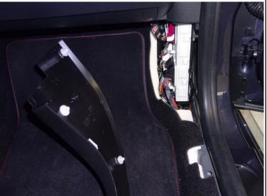
Connect the ring connector of the black REMUS power cable onto the vehicle ground.
