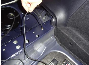
Wire the actuator cable along the car's chassis to the REMUS exhaust flap. Use cable ties to fix the cable into position!
