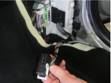
Connect the red wire of the REMUS power cable to the wire of PIN 20, by using the supplied connector!
