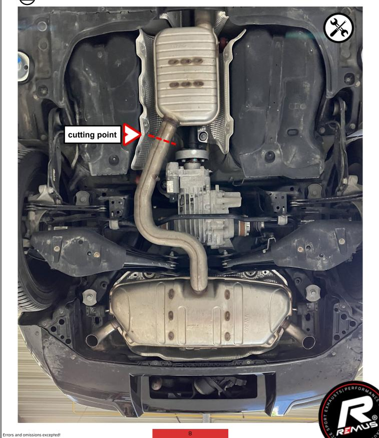
Unhook and unscrew the rubber hangers. Remove the stock exhaust.
