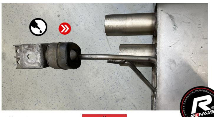
Install the REMUS connection tube on the original tube, use the supplied adapter.
