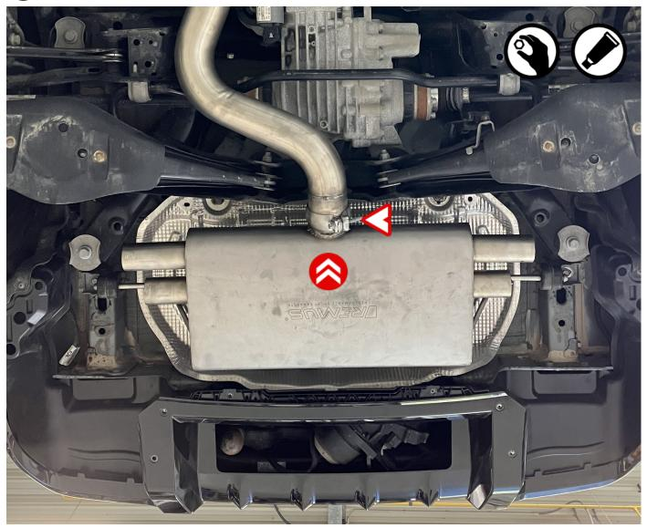
Remount the brackets onto the car body.
