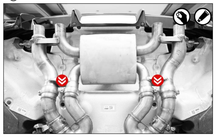
Remount the brackets onto the car's chassis.
