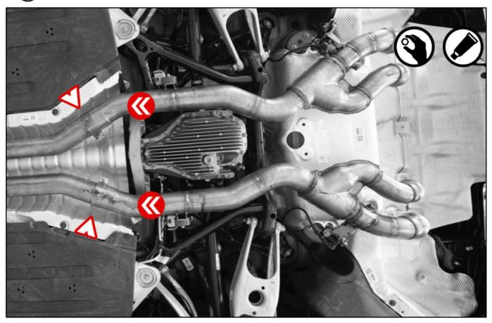
Mount the brackets onto the car's chassis and connect the actuators.
