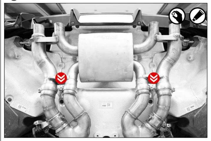
Remount the brackets onto the car's chassis.
