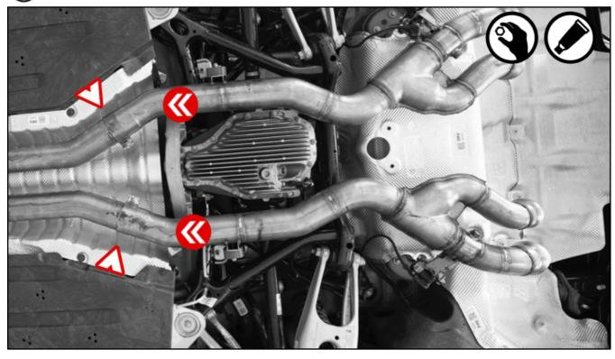
Mount the brackets onto the car's chassis and connect the actuators.
