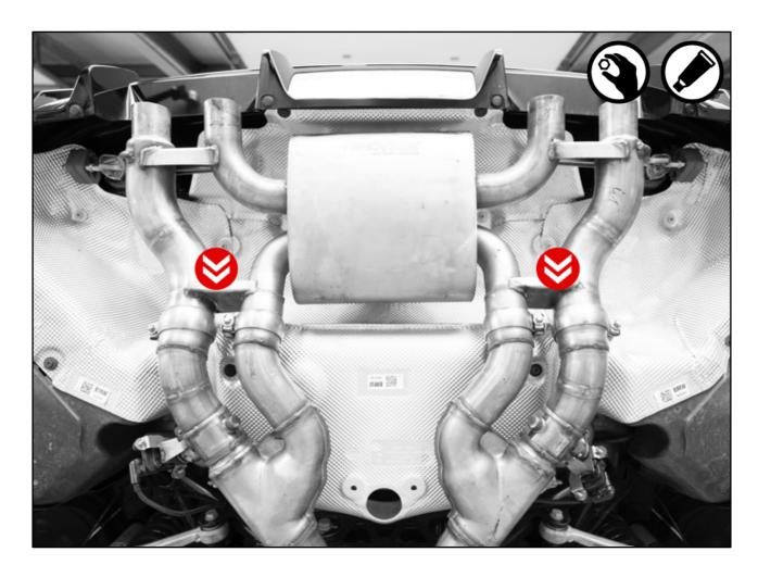
Remount the brackets onto the car's chassis.
