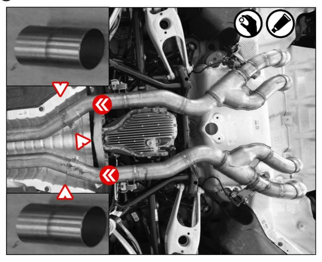
Mount the brackets onto the car's chassis and connect the actuators.
