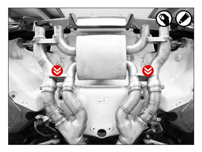
Remount the brackets onto the car's chassis.
