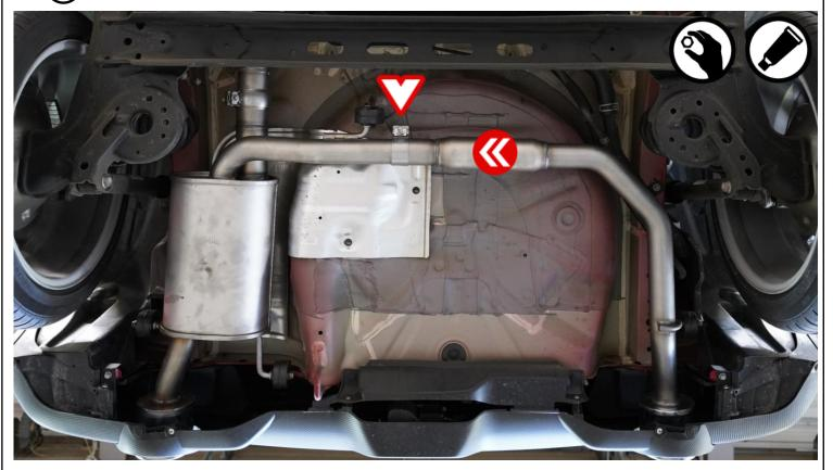
Remount the bracket onto the rubber hanger.
