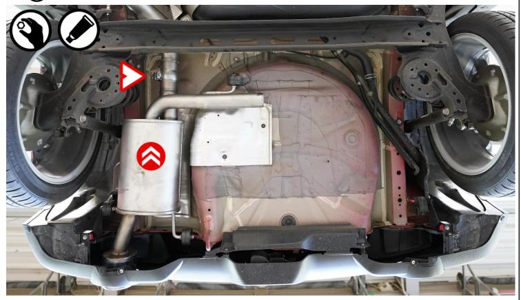
Remount the brackets onto the rubber hangers.
