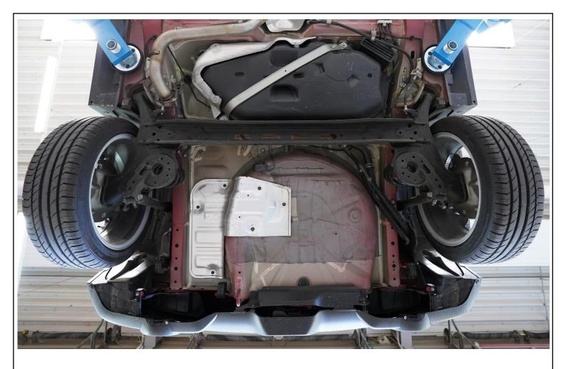
Unscrew the flange connection, unhook the rubber hanger and remove the standard front silencer.
