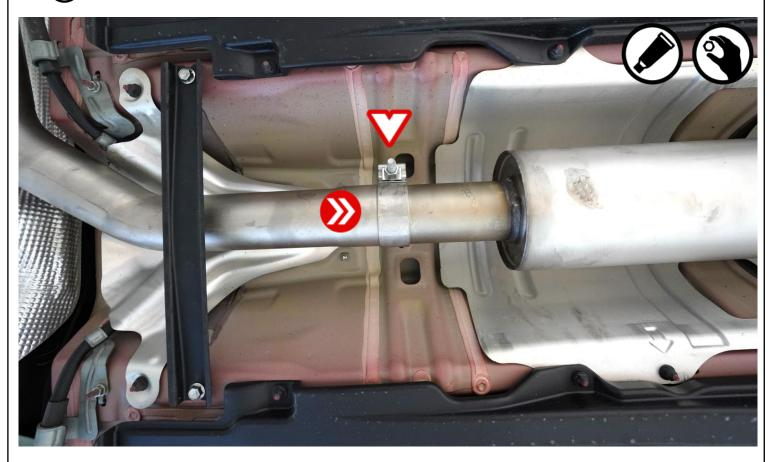
Remount the bracket onto the rubber hanger.
