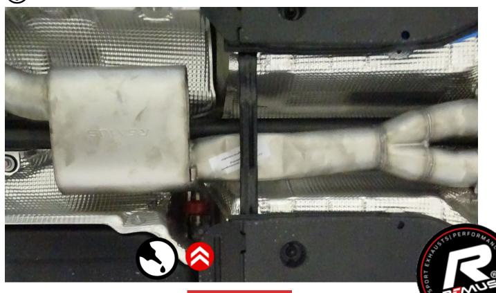
Install the REMUS connection tube on the front silencer. Hang in the rubber hanger.
