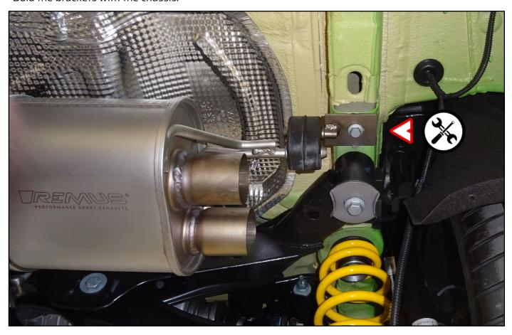
Mount the outlet tubes onto the sport exhaust.
