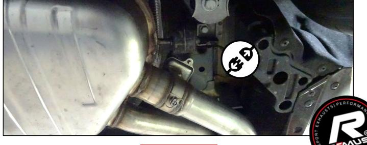
Unhook and unscrew the rubber hangers and remove the standard exhaust.
