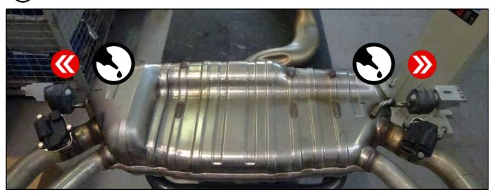
Mount the stock rubber hangers with the supplied REMUS chassis brackets onto the REMUS sport exhaust.
