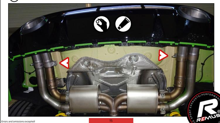
Align the exhaust system and tighten all connections.
