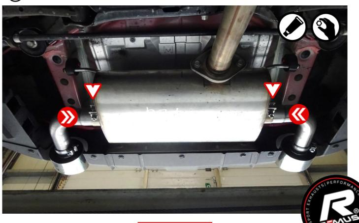
Align the exhaust system and tighten all connections.
