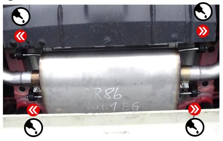
Slip on the outlet tube onto the sport exhaust. Use the supplied clamps.
