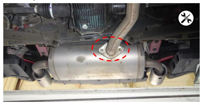
Unhook the rubber hangers and remove the standard exhaust.
